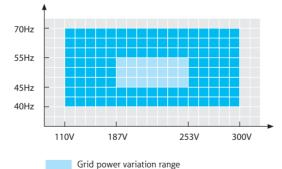
C1-3KVA wide input voltage and frequency range
